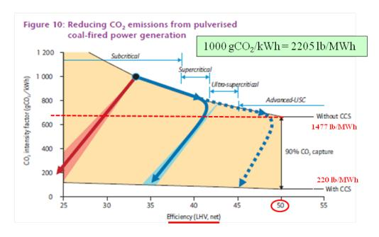
The Advanced Ultra Supercritical Pulverized Coal Plant(USCPC) at 1540 lb-CO<sub>2</sub>/MWh, would appear to meet the interim full load threshold level of 1534 lb-CO<sub>2</sub>/MWh, but another 15% efficiency improvement would be required to meet the final threshold of 1305 lb-CO<sub>2</sub>/MWh. Either that, or 15% Carbon Capture would be required.
